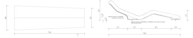
Construction Base: Rust-free metal Construction Base covering: Fibreglass Covering finish: Metallic lacquer
